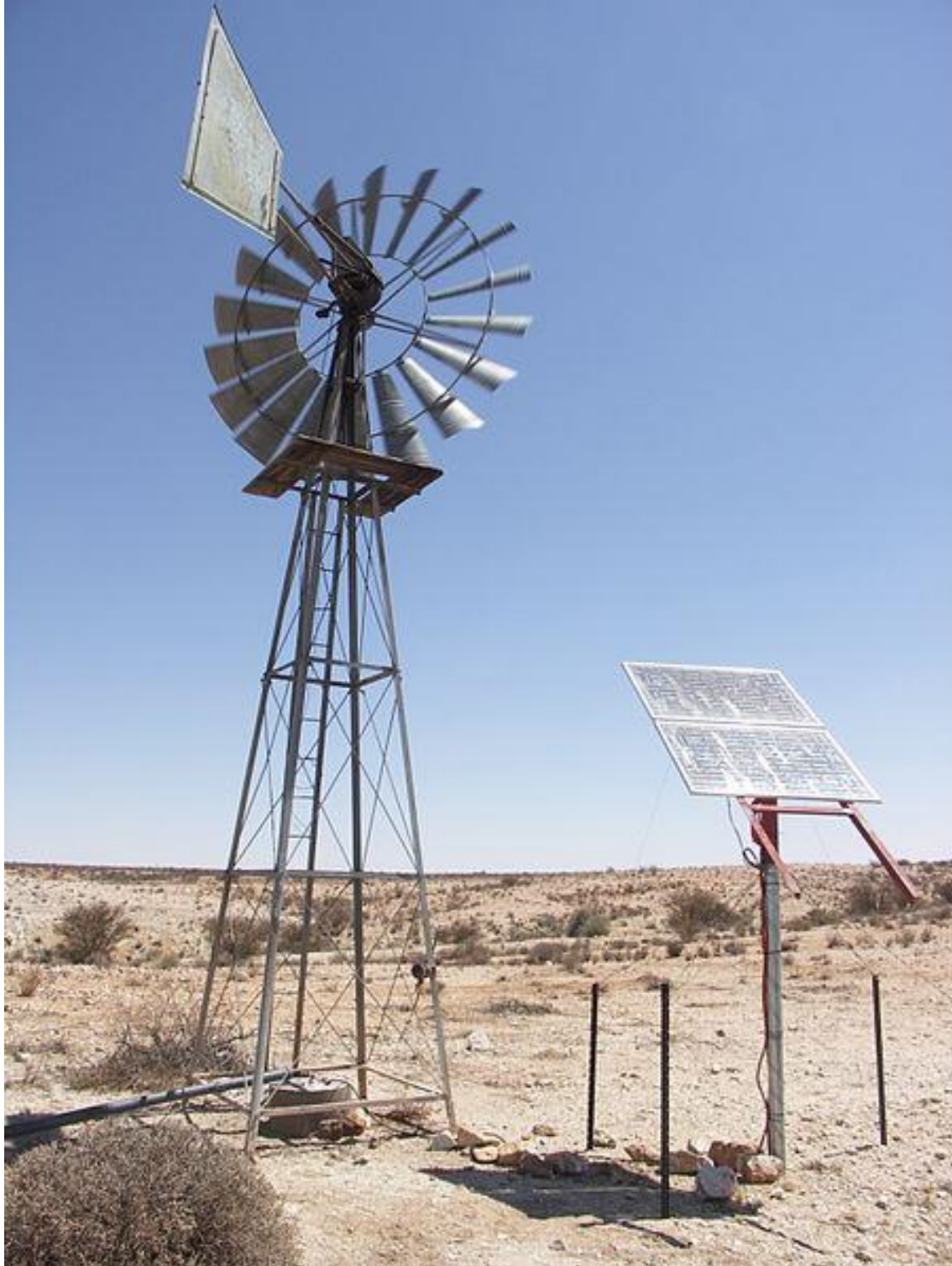
A windpump replaced by a solar powered pump at a water hole in the Augrabies Falls National Park.
